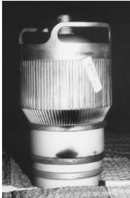
Figure 11. A4CX5000A tubes that appears to have suffered socketing problems.
